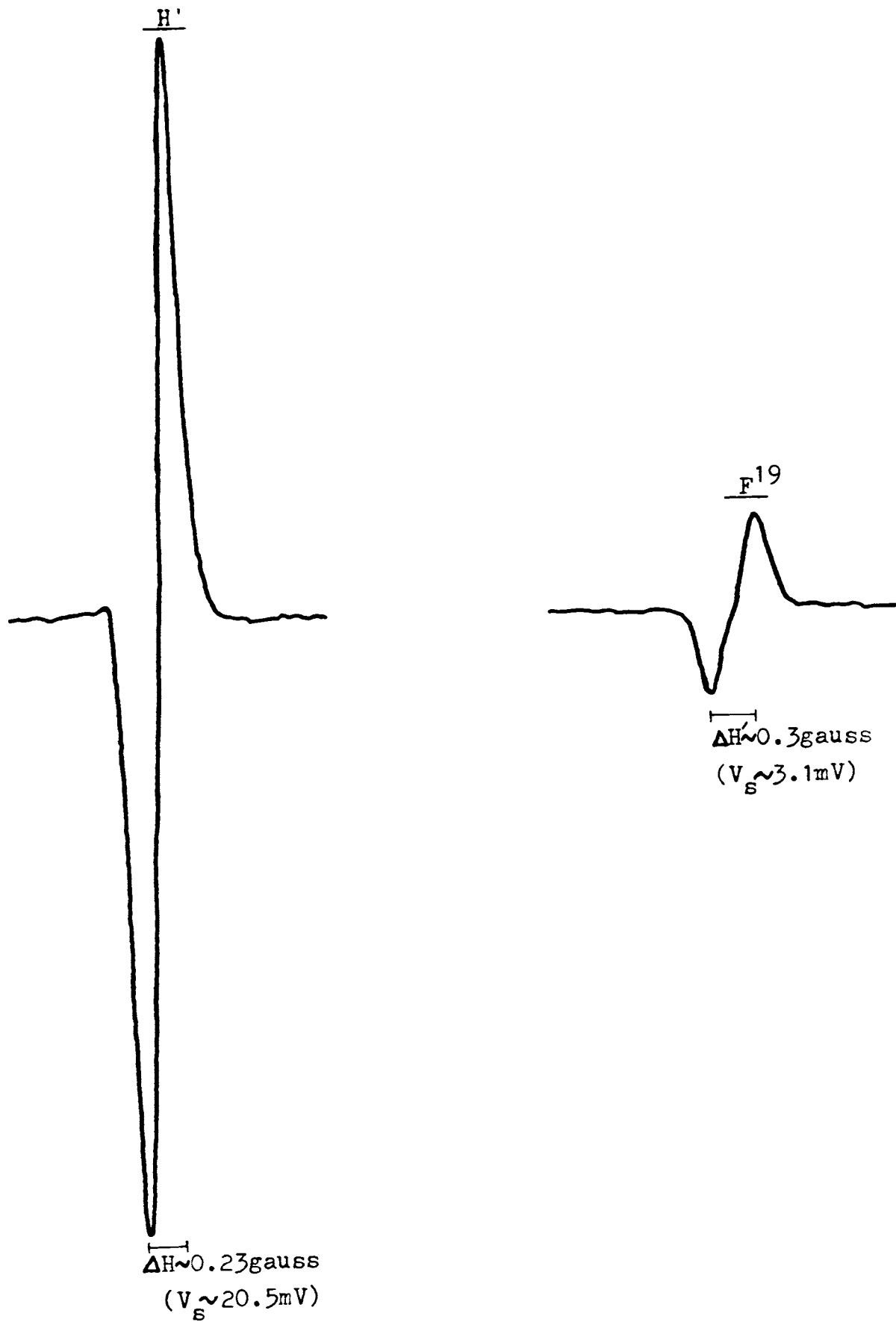
Fig. 7.2 : H^1 and F^{19} resonances from Hydro Fluoric acid
