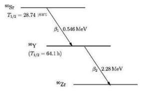
Strontium-90 is an isotope of strontium produced by the nuclear fission of uranium, having a radioactive half-life of 28.8 years. It undergoes  $\beta$ -decay transformed into yttrium-90 , with an energy of 0.546 MeV decay. the beta decay of strontium 90 gives rise to the emission of beta particles with maximum energy of 0,546MeV and 2,28Mev.
