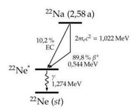
The isotope Na-22 decays (in 99.95% of cases) with a half-life of 2.6 years, by positron emission or electron capture to the first excited state of 22Ne 1,274 MeV (which then relaxes by emitting gamma photon). The positrons are emitted by the source at an energy of 544keV. When they annihilate, they produce two gamma photons of energy 0.511 MeV each.
