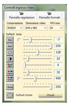
In order to obtain the best results it is advisable to set the Webcam with the parameters shown in the image aside. The following parameters are important:
