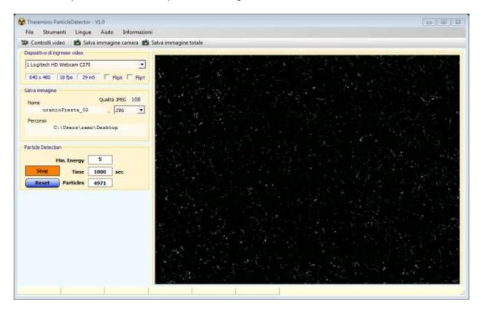
The application gives the possibility to set the **minimum energy (0 - 255)** in order not to count spurious events caused by the noise of CMOS sensor.
