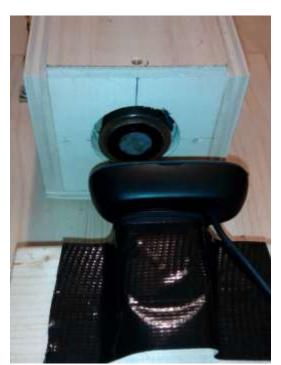
We used the Webcam sensor to do a test with a **15kV X-ray** generator. In the figure we see the detail of the Cam positioned in front of the front window (beryllium) of the tube. The Cam is sensitive, even if with low efficiency, to the X-ray. Below you see the detail of some pixels activated by X photons. The pixel brightness is low due to the low X photon energy.
