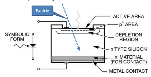
Actually the CMOS sensor is not optimized for the detection of the particles and therefore the detection efficiency is rather low, especially due to the fact that the sensitive region which is the depletion layer of the junction is very thin.
