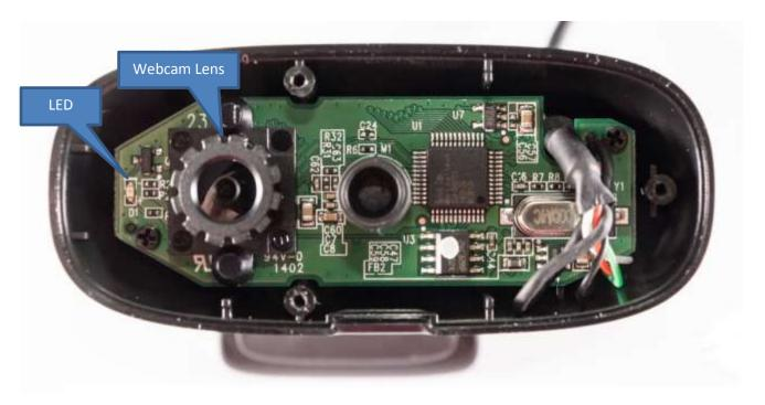
To prevent that the CMOS sensor is reached by LED light it is better to take it off with wire cutters or with solder. It should also be taken off even the webcam lens, as seen in the image below.
