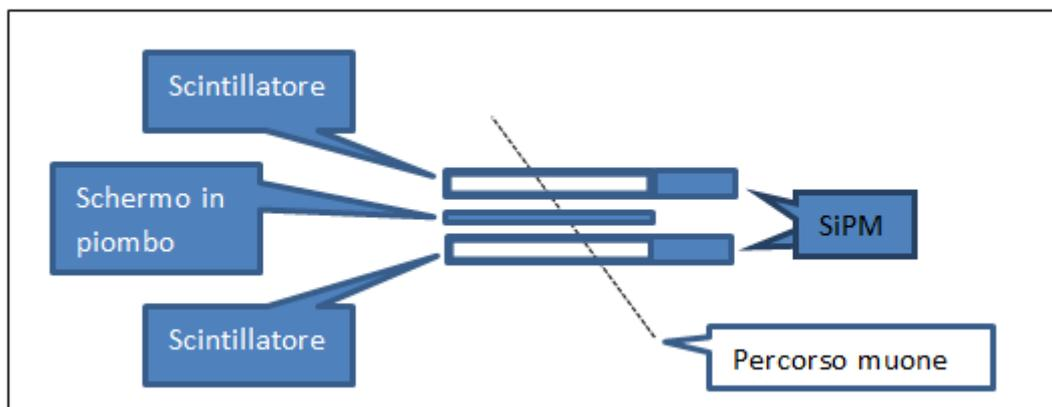
As seen in the figure above the two plastic scintillator crystals were placed one above the other and separated by a lead screen to stop environmental radiation.
