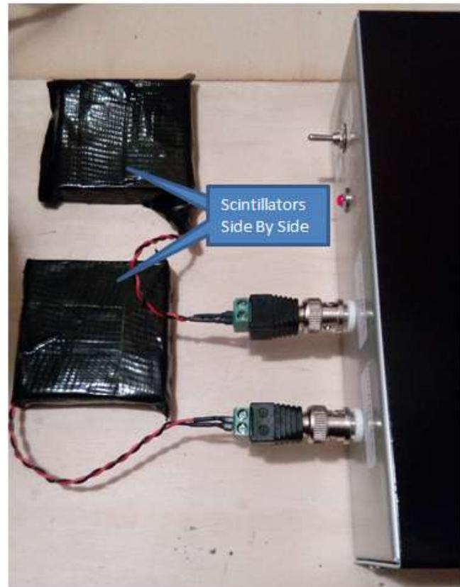
The pulses from SiPM are sent to an electronic device that performs the shaping of the pulses and produces the coincidence pulse with an AND logic gate :
