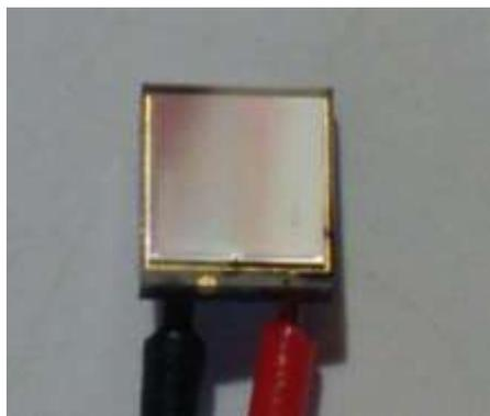
The SiPM sensor has been placed on a side of the scintillator crystal and fixed with transparent adhesive tape, to increase the optical coupling efficiency, between the SiPM and the crystal a layer of silicon Optical grease has been spread :
