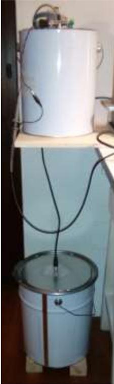
By using the Cherenkov detector and the plastic scintillator it has been made a setup for the detection of coincident pulses.
