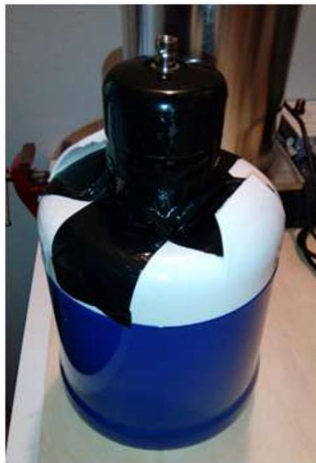
To reduce internal reflections the PMT was placed so that the photo-cathode is immersed within the water. Water must be distilled and purified so that internal absorption inside the liquid is minimized.
