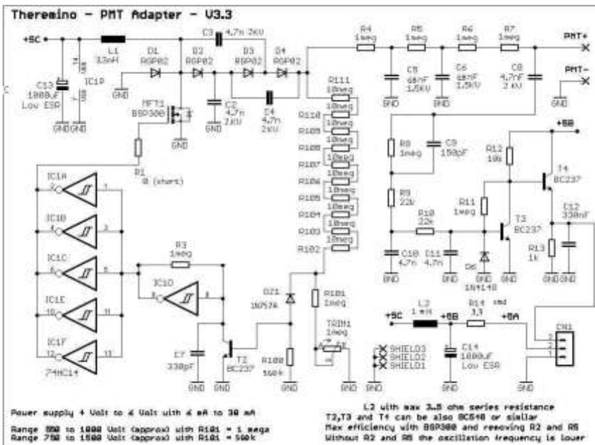
The photomultiplier tube is fed by means of a Theremino PMT adapter placed inside the metal container. Actually it is used only the high voltage generation part. The signal is taken from the capacitor C8, while the entire part of " pulse shaping " has not been assembled. The HV driver power supply is via 5V low voltage, which can be easily provided by a series of 4 1,5V batteries, the voltage can be reduced a bit with a diode connected in series.
