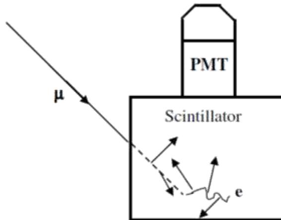
**Schematic showing the generation of the two light pulses (short arrows) used in determining the muon lifetime. One light pulse is from the slowing muon (dotted line) and the other is from its decay into an electron or positron (wavy line)**
