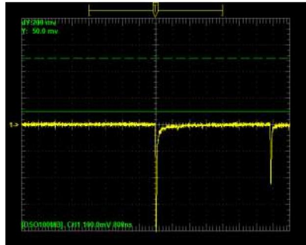
**Examples of pulses caused by the passage of a muon and the subsequent decay into an electron. The electron has high kinetic energy, and then leaves a trace of amplitude similar to that of the muon. In the first case the time interval is approximately 1600ns, in the second case approximately 5600ns.**
