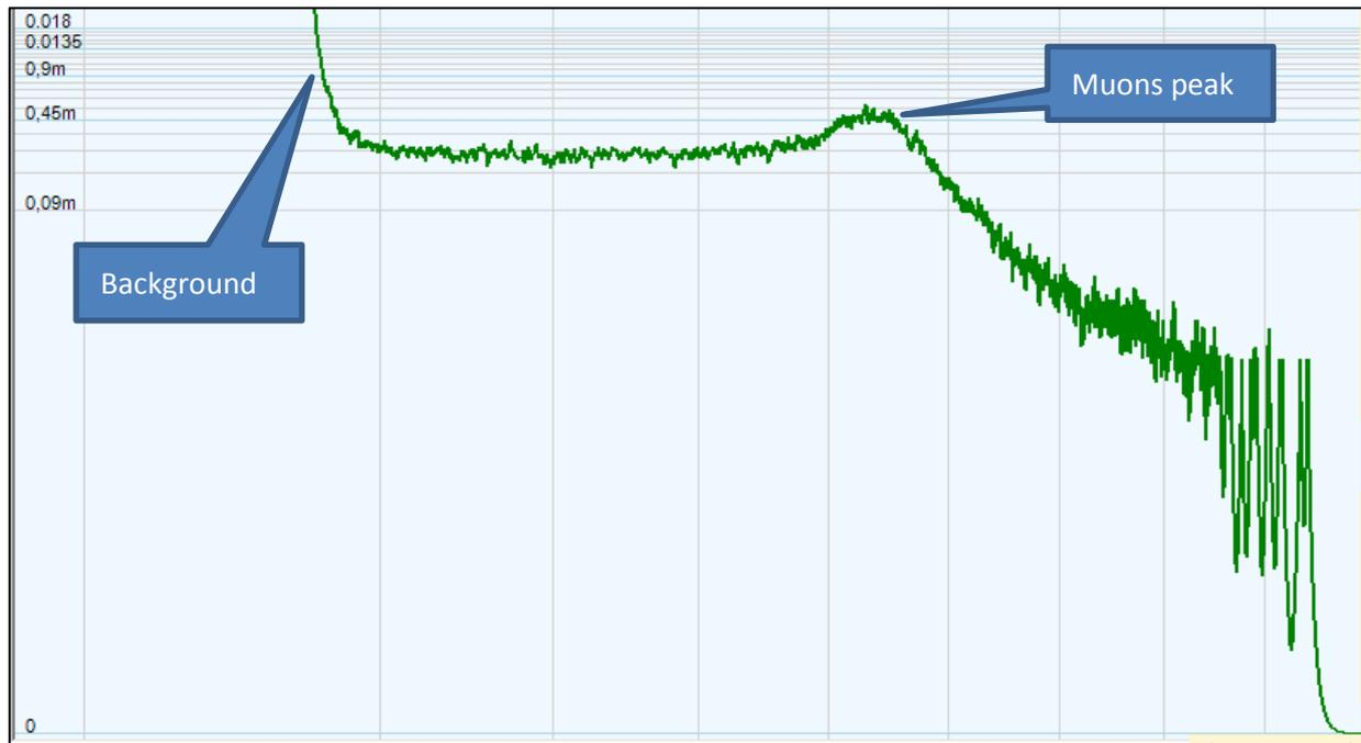
**Spectrum obtained with a software MCA in which it is shown the peak at high energies due to the absorption of muons in the plastic scintillator crystal .
