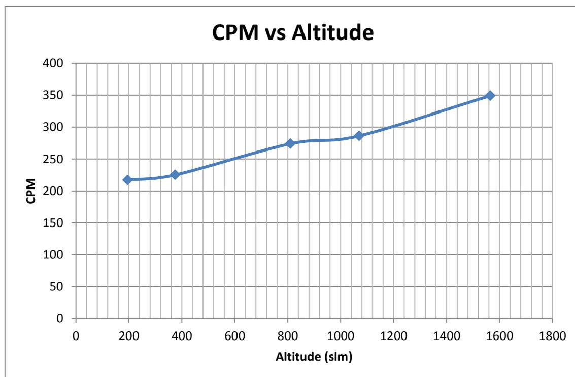
Chart showing the muon flux at different altitudes. It is clear that the more the altitude the higher the muon flux value. The increase of the altitude increases the flow because it decreases the thickness of atmosphere traversed by the muons and therefore it reduces the likelihood of absorption and spontaneous decay.
