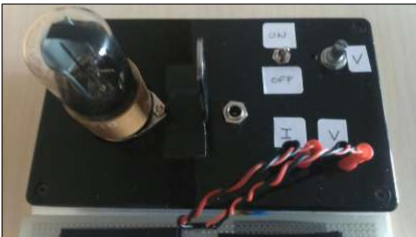
Phototube, potentiometer and pins for connections of measurement of stopping voltage and photocurrent
