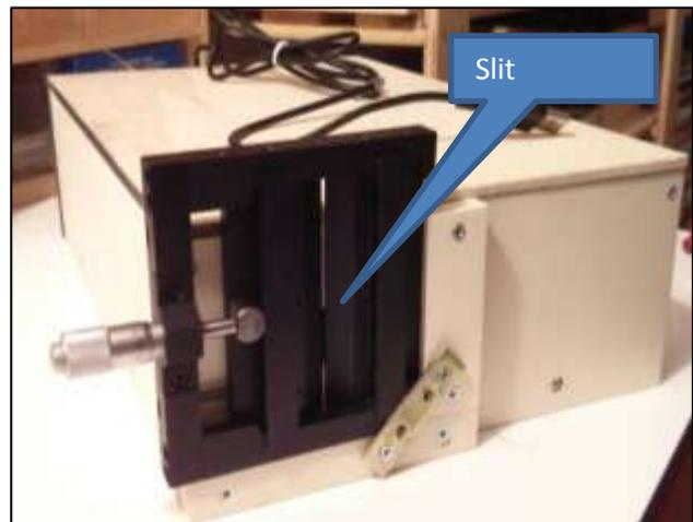
Detail of the micrometric slit and the spectrometer assembled
