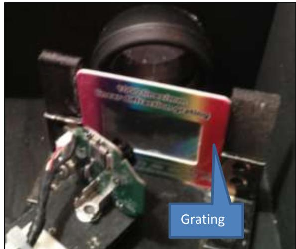
Inside view with collimating lens, grating and webcam
