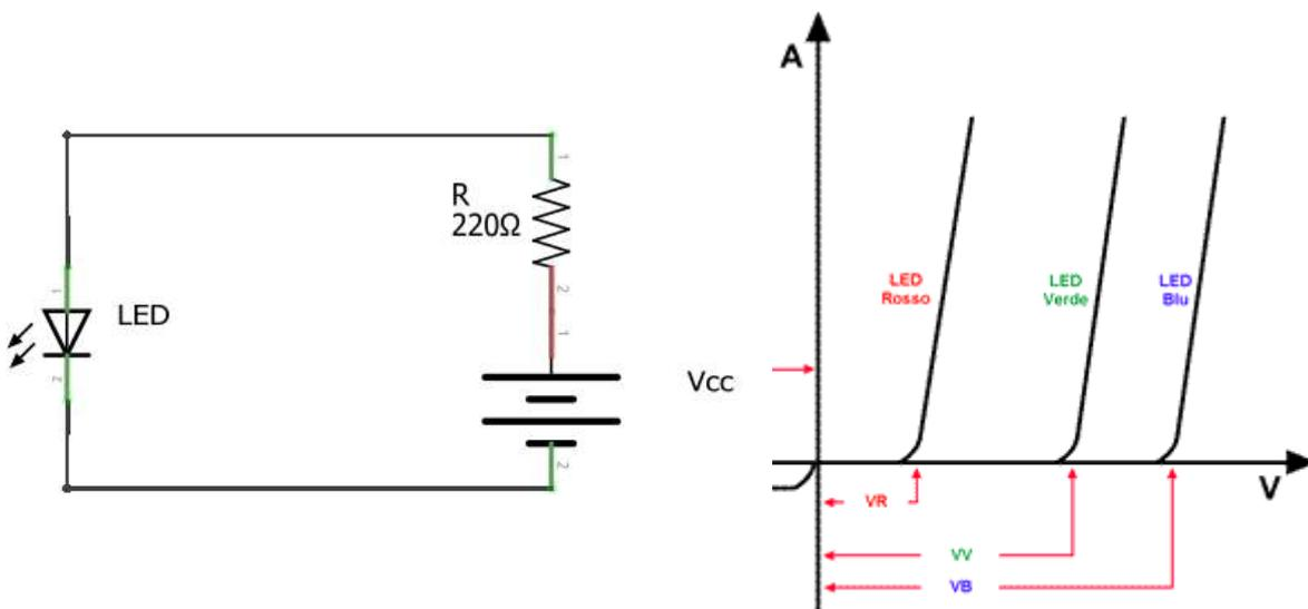
The activation voltage of the LED is determined by measuring the voltage that occurs across the diode LED when the LED starts to emit light. In order to accurately determine this voltage value the test was done in a darkened room.
